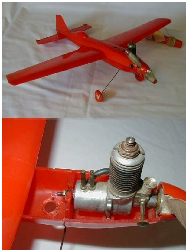
Baby Spitfire powered Aeromite, details unknown Note the 2 long filler tubes and central mounting bolt
